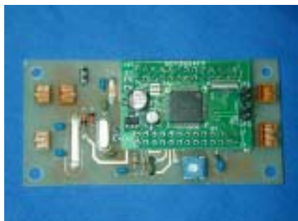
Fig. 13 Terminal Node Controller (TX/RX)
