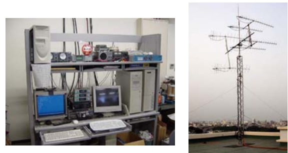
Fig. 1 Ground Station System
