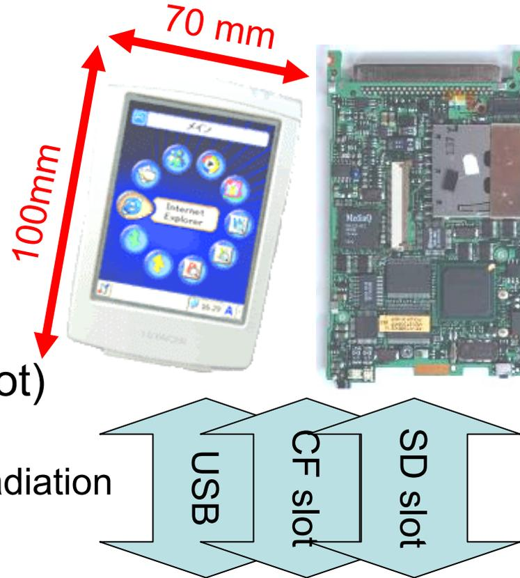
This PDA is good tolerant performance on radiation test at Osaka University In July 2004.
