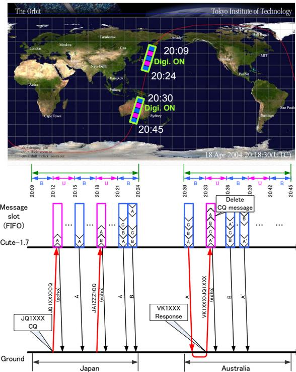
Fig. 4 Communication Example Using Digital Repeater
