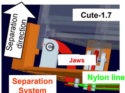
Fig. 12 Mechanism of Separation
