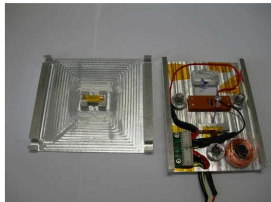
Fig.7 Tether Deployment Mechanism
