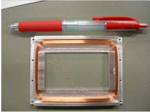
Fig.3 Magnetic Torquer
