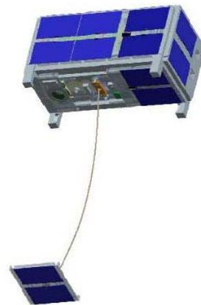
Fig.6 Image of Tether Deployment Experiment
