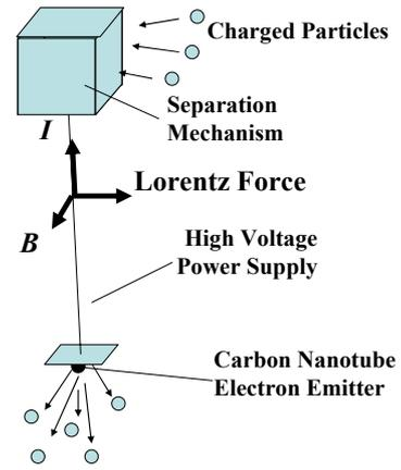
Fig.5 Tether Deorbit System
