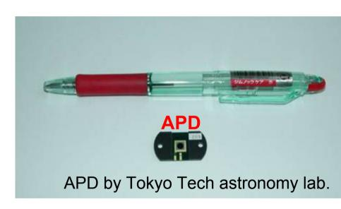
Measure Low-E(E>3 kev) e-/p distributions in SAA and aurora band APD will be installed on the future large X-ray astronomy satellite.
