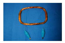
Fig.4 Prototype of Magnetic Torquer
