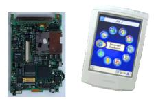
Fig.2 Hitachi PDA NPD-20JWL internal circuit board(right), external view(left)
