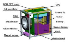
(b) Equipment Layout Fig.11 TSUBAME satellite
