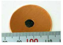
Fig.6 Prototype of Carbon-nano-tube Emitter
