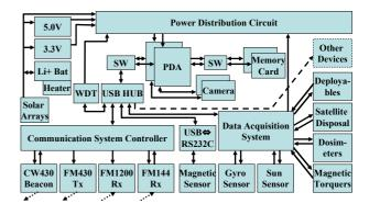
Fig.3 System Block Diagram
